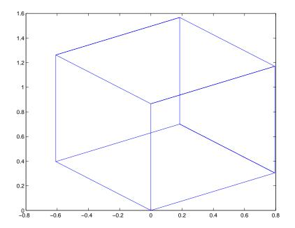
Use a perspective transformation with a 25 degree viewing angle:
