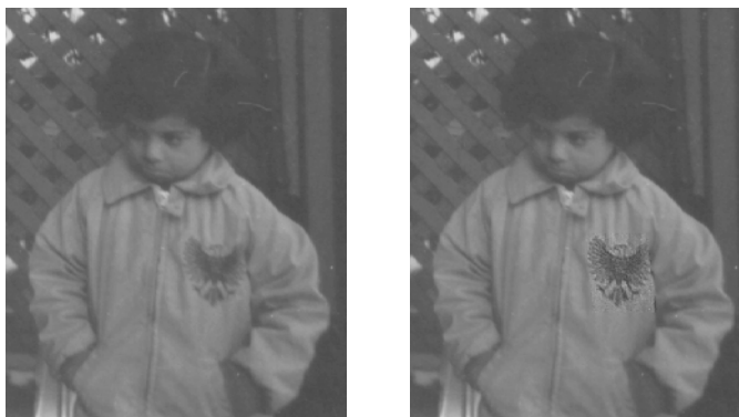
Image Before and After Using an Unsharp Filter on the Region of Interest
