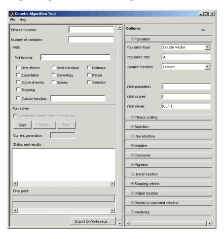
You can use the Genetic Algorithm Tool to run the genetic algorithm on optimization problems and display the results. See "Using the Genetic Algorithm Tool" on page 2-4 for a complete description of the tool.
