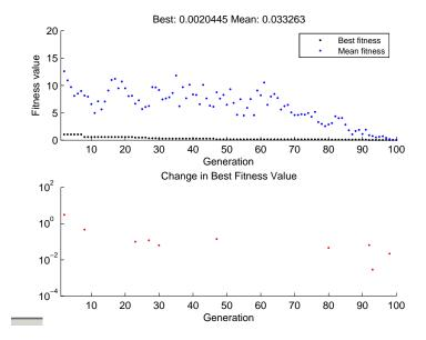
Note that because the scale of the y-axis in the lower custom plot is logarithmic, the plot only shows changes that are greater then 0. The logarithmic scale enables you to see small changes in the fitness function that the upper plot does not reveal.
