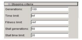
When you run the genetic algorithm, the **Status** panel displays the criterion that caused the algorithm to stop.
