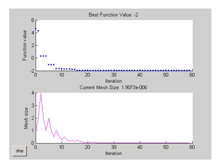
The upper plot displays the objective function value at each iteration. The lower plot displays the coordinates of the point with the best objective function value at the current iteration.
