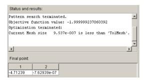
The minimum function value is approximately -2. The **Final point** pane displays the point at which the minimum occurs.
