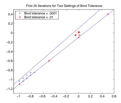
Note that when **Bind tolerance** is set to .01, the points move toward the optimal point more quickly. The pattern search requires only 90 iterations. When **Bind tolerance** is set to .0001, the search requires 124 iterations. However, when the feasible region does not contain very acute angles, as it does in this example, increasing **Bind tolerance** can increase the number of iterations required, because the pattern search tends to poll more points.
