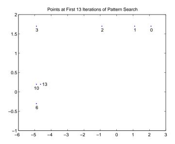
The numbers below the points indicate the first iteration at which the algorithm finds the point. The plot only shows iteration numbers corresponding to successful polls, because the best point doesn't change after an unsuccessful poll. For example, the best point at iterations 4 and 5 is the same as at iteration 3.
