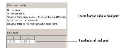
You can change many of the settings in the Genetic Algorithm Tool while the algorithm is running. Your changes are applied at the next generation. Until your changes are applied, which occurs at the start of the next generation, the **Status and Results** pane displays the message Changes pending. At the start of the next generation, the pane displays the message Changes applied. as shown in the following figure.
