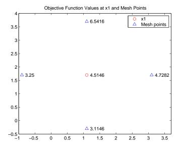
The algorithm polls the mesh points until it finds one whose value is smaller than 4.5146, the value at x1. The first such point it finds is [-0.9 1.7], at which the value of the objective function is 3.25, so the poll at iteration 2 is again successful. The algorithm sets the second point in the sequence equal to
