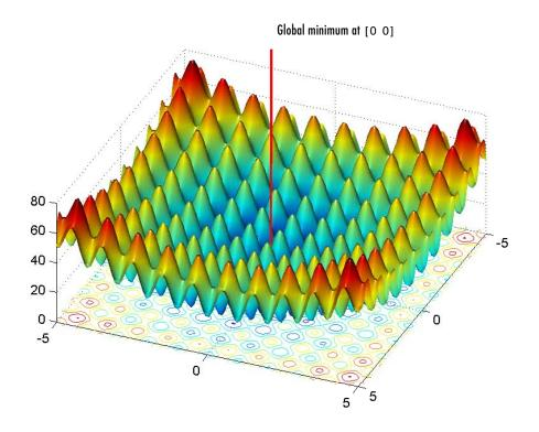
As the plot shows, Rastrigin's function has many local minima — the "valleys" in the plot. However, the function has just one global minimum, which occurs at the point  $[0\ 0]$  in the x-y plane, as indicated by the vertical line in the plot, where the value of the function is 0. At any local minimum other than  $[0\ 0]$ , the value of Rastrigin's function is greater than 0. The farther the local minimum is from the origin, the larger the value of the function is at that point.
