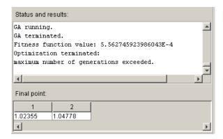
The final point is close to the true minimum at (1, 1). You can improve this result by setting **Hybrid function** to fminunc in **Hybrid function** options.
