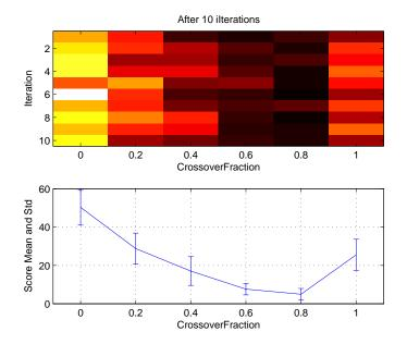
The lower plot shows the means and standard deviations of the best fitness values over 10 generations, for each of the values of the crossover fraction. The upper plot shows a color-coded display of the best fitness values in each generation.
