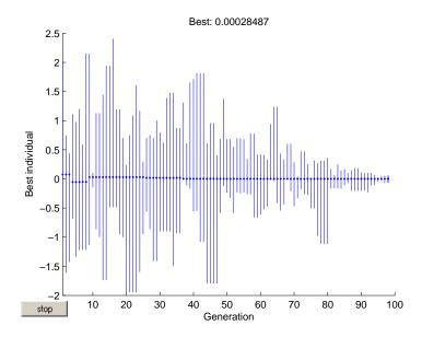
Note that all individuals are between -2 and 2.5. While this range is larger than the default Initial range of [0;1], due to mutation, it is not large enough to explore points near the global minimum at x = 21.
