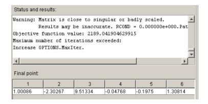
The algorithm halts because it exceeds the maximum number of iterations, whose value you can set in the **Max iteration** field in the **Stopping criteria** options. The default value is 100 times the number of variables for the objective function, which is 6 in this example.
