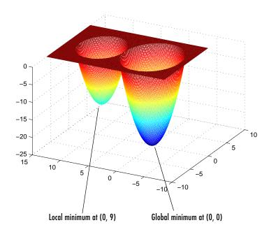
The global minimum of the function occurs at (0, 0), where its value is -25. However, the function also has a local minimum at (0, 9), where its value is -16.
