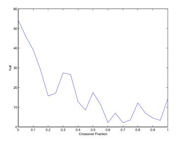
The plot indicates that you get the best results by setting options.CrossoverFraction to a value somewhere between 0.6 and 0.95. You can get a smoother plot of fval as a function of the crossover fraction by running ga 20 times and averaging the values of fval for each crossover fraction. The following figure shows the resulting plot.
