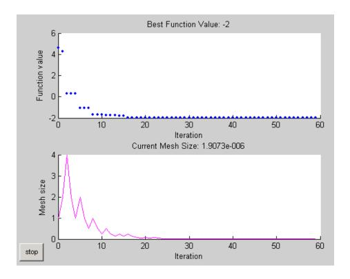
The upper plot shows the objective function value of the best point at each iteration. Typically, the objective function values improve rapidly at the early iterations and then level off as they approach the optimal value.
