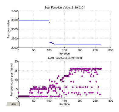
To see the effect of using a search method, select Positive Basis Np1 in the **Search method** field in **Search** options. This sets the search method to be a pattern search using the pattern for Positive basis Np1. Then click **Start** to run the genetic algorithm. This displays the following plots.
