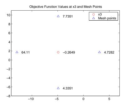
At this iteration, none of the mesh points has a smaller objective function value than the value at x3, so the poll is *unsuccessful*. In this case, the algorithm does not change the current point at the next iteration. That is,
