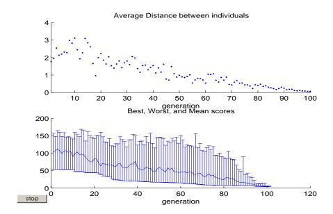
The upper plot displays the average distance between points in each generation. As the amount of mutation decreases, so does the average distance between individuals, which is approximately 0 at the final generation. The lower plot displays a vertical line at each generation, showing the range from the smallest to the largest fitness value, as well as mean fitness value. As the amount of mutation decreases, so does the range. These plots show that
