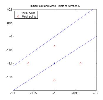
The top mesh point, which is (-1.001, -1.0375), has a smaller objective function value than the initial point, so the poll is successful.
