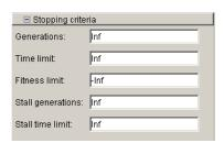
**Note** Do not use these settings when calling the genetic algorithm function ga at the command line, as the function will never terminate until you press **Ctrl + C**. Instead, set **Generations** or **Time** limit to a finite number.
