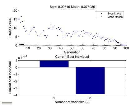
The upper plot displays the best and mean fitness values in each generation. The lower plot displays the coordinates of the point with the best fitness value in the current generation.
