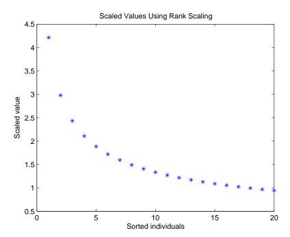
The following plot shows the scaled values of the raw scores using rank scaling.
