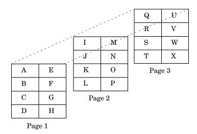
MATLAB internally represents the data for this three-dimensional array in the order shown below:
