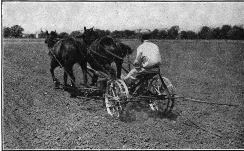
FIG. 19. Two-row corn planter checking corn that is planted so that the cross rows drop by means of a wire at straight right angles to the forward motion of the planter.
