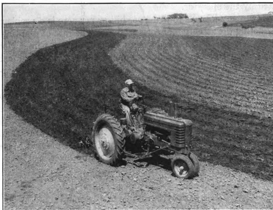
FIG. 21. Two-row integral lister, planting corn on contour. (Courtesy John Deere Plow Co.)
