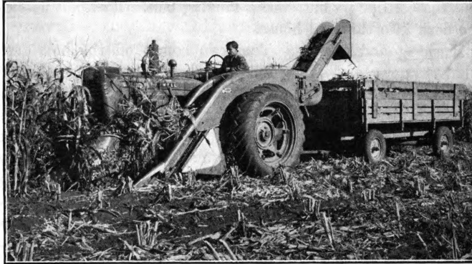
FIG. 44. A mechanical corn picker which cuts the stocks loose from the ground, delivers the ears to the trailer wagon, and shreds the fodder before spreading it on the ground. This type of machine is effective in destroying most of the corn borers which are in the stocks that are shredded. The illustration shows the machine without the snapping rollers and husking attachments, harvesting sweet corn for canning.
