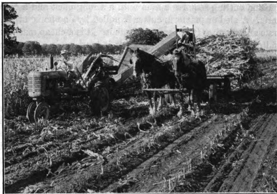
FIG. 38. Corn binder in the field with loader attachment delivering bundles to the wagon. (Courtesy International Harvester Co.)
